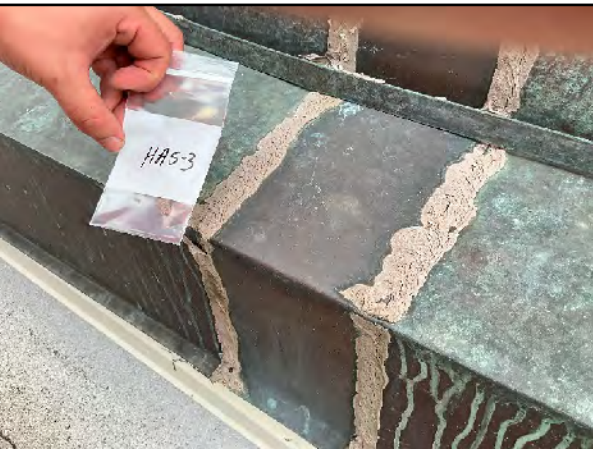
Figure (17) – Asbestos Bulk Sample HA5-3 – Tan Caulk at Brick Stack.
