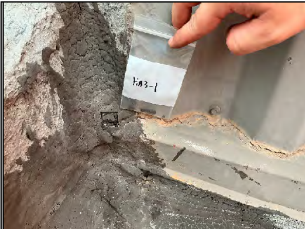
Figure (9) – Asbestos Bulk Sample HA3-1 – Black Mastic at Penetrations.
