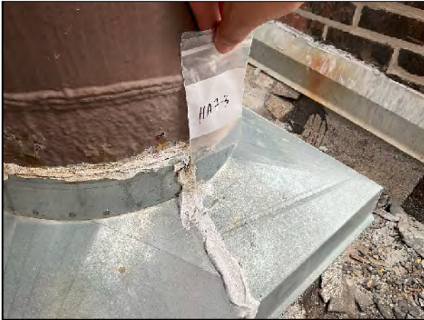
Figure (25) – Asbestos Bulk Sample HA7-3 – Gray Caulk at Penetrations.
