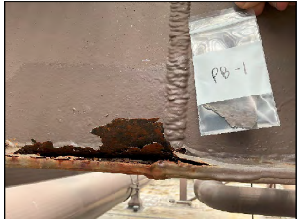
Figure (26) – Lead Bulk Sample PB-1 – Steel Girder and Pipes.
