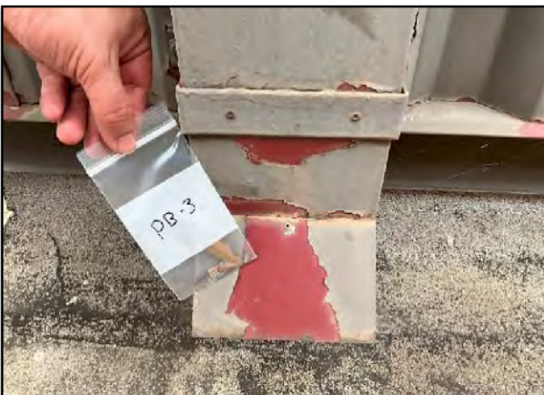
Figure (29) – Lead Bulk Sample PB-3 – Gray on building.
