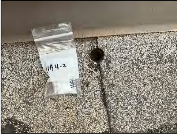
Figure (13) – Asbestos Bulk Sample HA4-2 – Flashing at Parapet Walls and Curbs.
