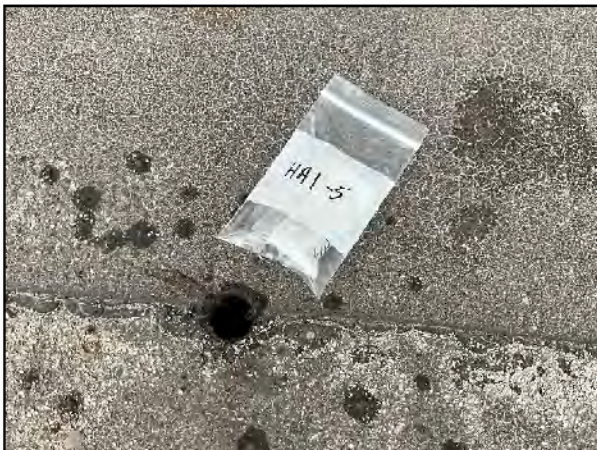
Figure (5) – Asbestos Bulk Sample HA1-5 – Original Gray Built Up Roofing (wet).
