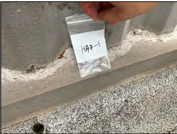
Figure (23) – Asbestos Bulk Sample HA7-1 – Gray Caulk at Penetrations.
