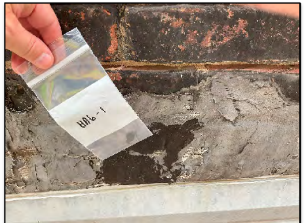
Figure (18) – Asbestos Bulk Sample HA6-1 – ACM Mastic from brick parapet wall at Northeast corner of c1920s Building.
