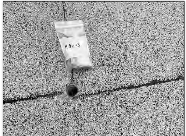
Figure (8) – Asbestos Bulk Sample HA2-3 – Newer Gray Built Up Roofing.
