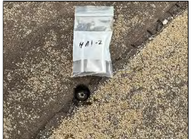
Figure (2) – Asbestos Bulk Sample HA1-2 – Original Gray Built Up Roofing.
