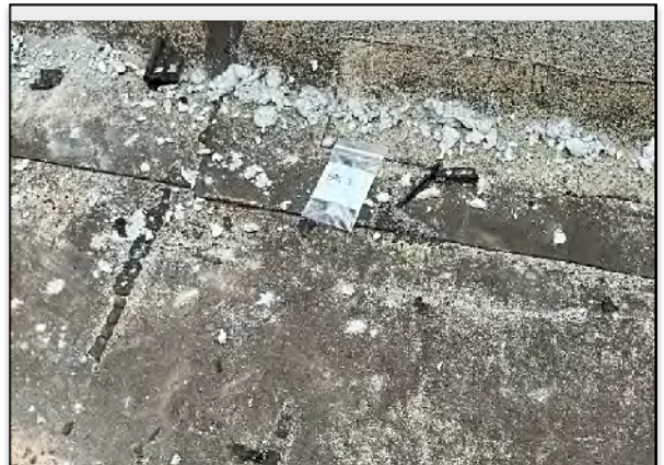
Figure (20) – Asbestos Bulk Sample HA6-2 – ACM Mastic from debris pile along East parapet wall of c1920s Building.
