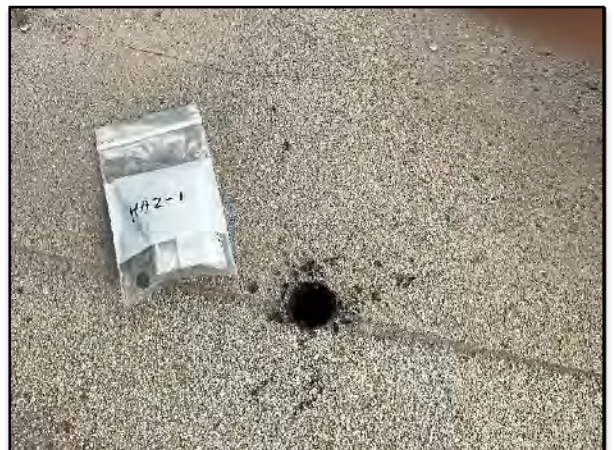
Figure (6) – Asbestos Bulk Sample HA2-1 – Newer Gray Built Up Roofing.
