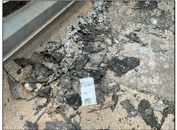
Figure (20) – Asbestos Bulk Sample HA6-2 – ACM Mastic from debris pile along East parapet wall of c1920s Building.
