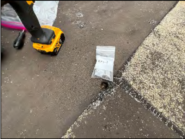
Figure (1) – Asbestos Bulk Sample HA1-1 – Original Gray Built Up Roofing.
