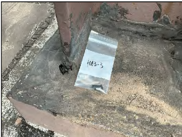
Figure (11) – Asbestos Bulk Sample HSA3-3 – Black Mastic at Penetrations.
