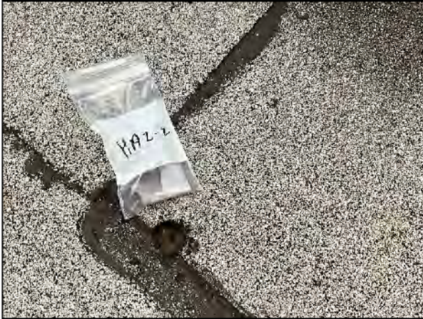
Figure (7) – Asbestos Bulk Sample HA2-2 – Newer Gray Built Up Roofing.
