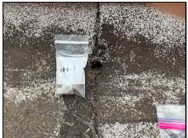
Figure (12) – Asbestos Bulk Sample HA4-1 – Flashing at Parapet Walls and Curbs.
