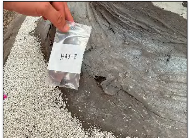
Figure (10) – Asbestos Bulk Sample HA3-2 – Black Mastic at Penetrations.
