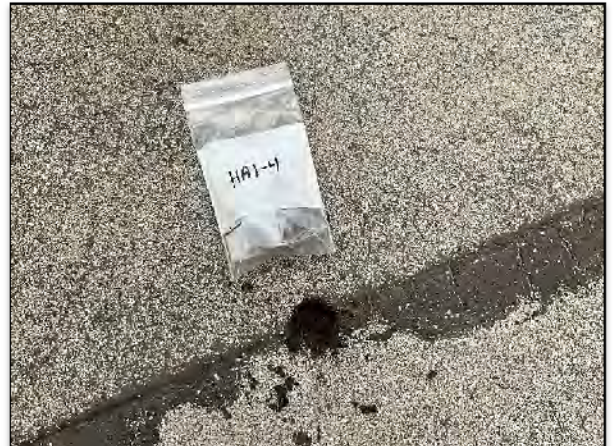
Figure (4) – Asbestos Bulk Sample HA1-4 – Original Gray Built Up Roofing.
