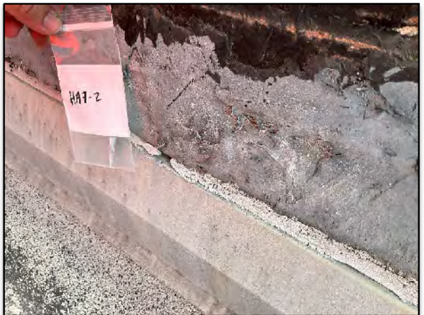
Figure (24) – Asbestos Bulk Sample HA7-2 – Gray Caulk at Penetrations.
