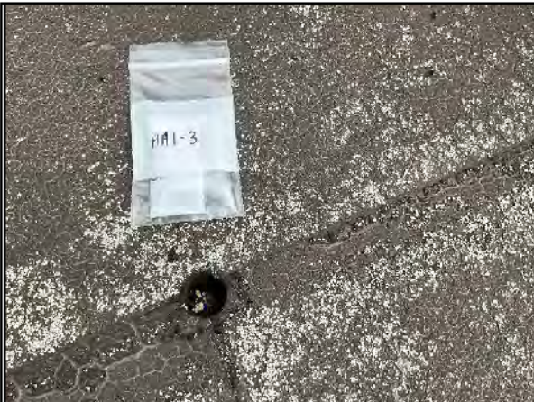
Figure (3) – Asbestos Bulk Sample HA1-3 – Original Gray Built Up Roofing.
